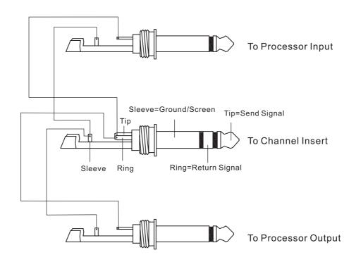
Y-Stereo lead for insert Connection
